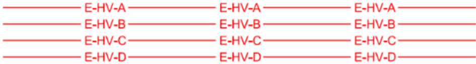
Figure 1: Example of appropriate line styles to indicate the verification of buried services.
